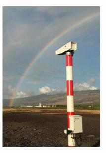
The TAA and MOR values are determined by the measurement of the dimming of a LED based white source (modulated at 30 Hz) through the atmospheric layer between the transmitter and the receiver.
